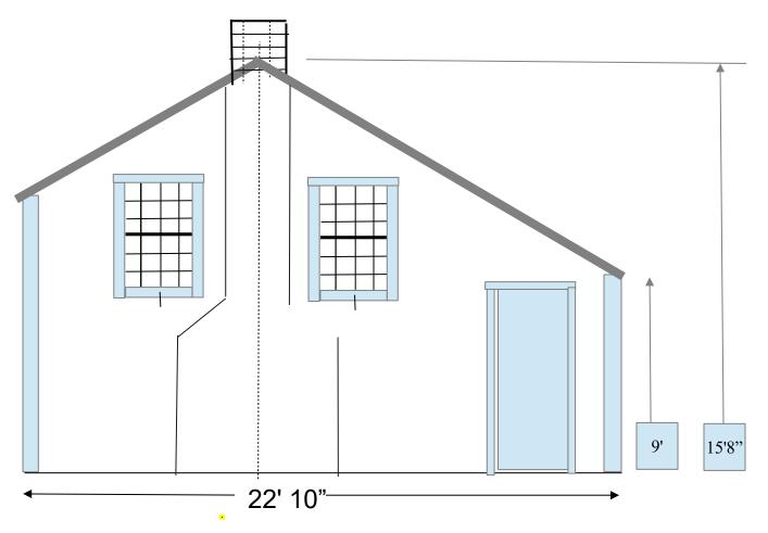
Rough chimney interior outline. Moving the Door to the north-west corner (from NE Corner). Windows would be 12/12's as with east wall, approximately 60" above floor height....
