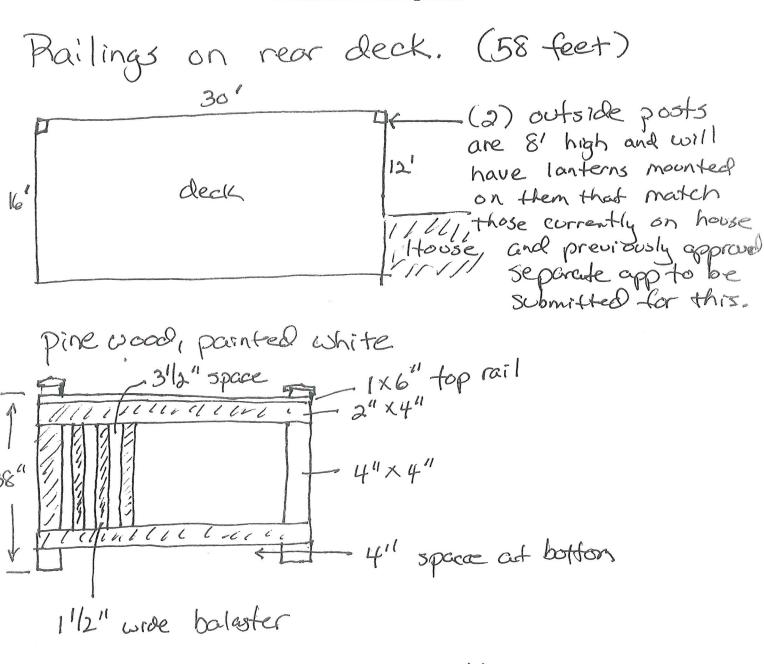
all attached of deck screws, not visible,
